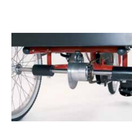
864 disc BRAKE applicable only on the models with differential (207 -3D, -4D and -5D)
